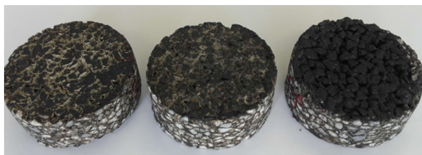
Fig. 1. Porous asphalt drill cores from different 2.5 m 2 porous asphalt samples (exemplary for PA 8 from left to right: soiled with 1440 g/m 2 ; soiled with 480 g/m 2 ; unsoiled/new).
