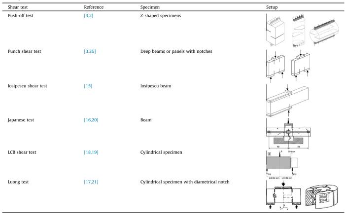
The assessment of pure shear behaviour of concrete is a complex task. No standardized tests are available and most of the tests found in the literature require special sample preparation and setups hardly compatible with the execution of SC structures. The selection and adaptation of a simple shear test to these conditions might represent an additional contribution since the results obtained could be used for the quality control of the variability of the material.
