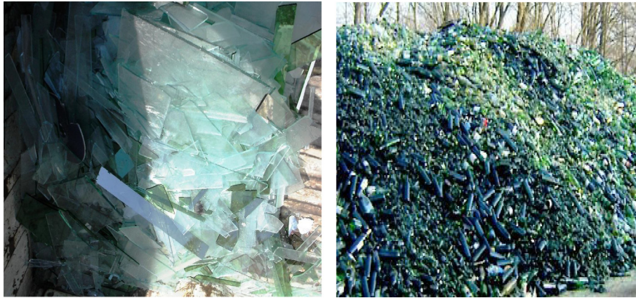
Fig. 1. Wastes of glass in solid form resulted from crushed containers and construction demolishing in Egypt.
