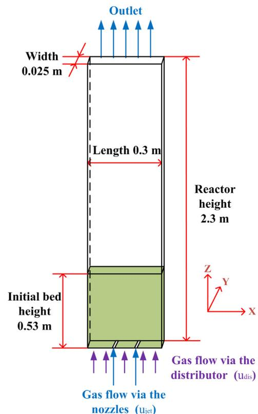
Fig. 1. Sketch of the rectangular two-jet fluidized bed.
