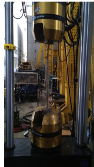
Fig. 2. Typical failure of BFRP rod.
