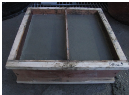
(a) Existing OPC concrete for pull-off test
