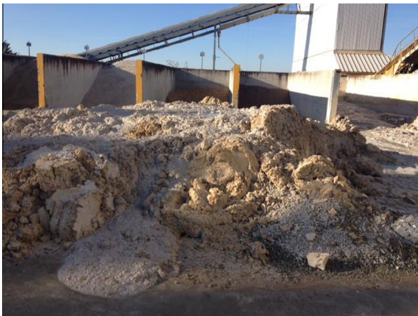
Fig. 1. Picture of the raw materials coming from the C4 ready-mixed concrete plant.
