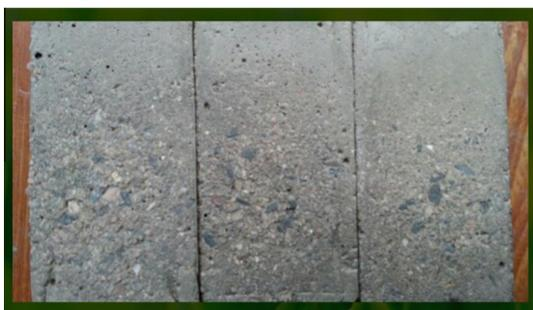
Fig. 1. Concrete specimens after erosion (from left to right C20, C30, C40).
