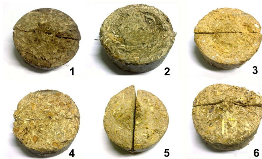
Fig. 1. Samples of the biomass briquettes examined (except cereal straw): (1) vine shoots, (2) rape straw, (3) rice husk, (4) maize stalk, (5) sawdust and cereal straw, and (6) maize stalk mixed with pine wood chips.
