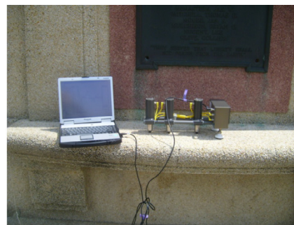
(b) PSPA test equipment
