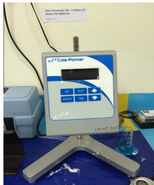
Fig. 2. Digital Brookfield Viscometer for epoxy resin viscosity test.
