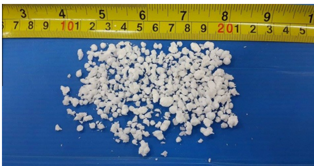
Fig. 1. Lightweight aggregates from recycled foam.
