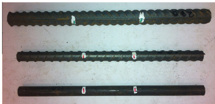
Fig. 2. Low-cycle fatigue test specimens.
