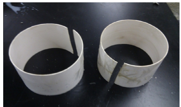
Fig. 2. The moulds of the test specimens.
