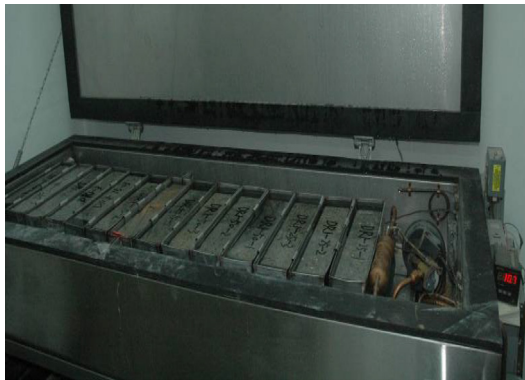
(a) Automatic quick concrete freeze-thaw tester
