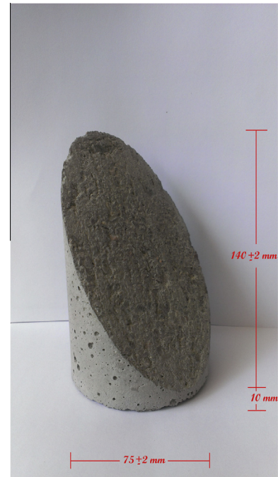
Fig. 1. Dimension of semi-specimens according to ASTM C882.
