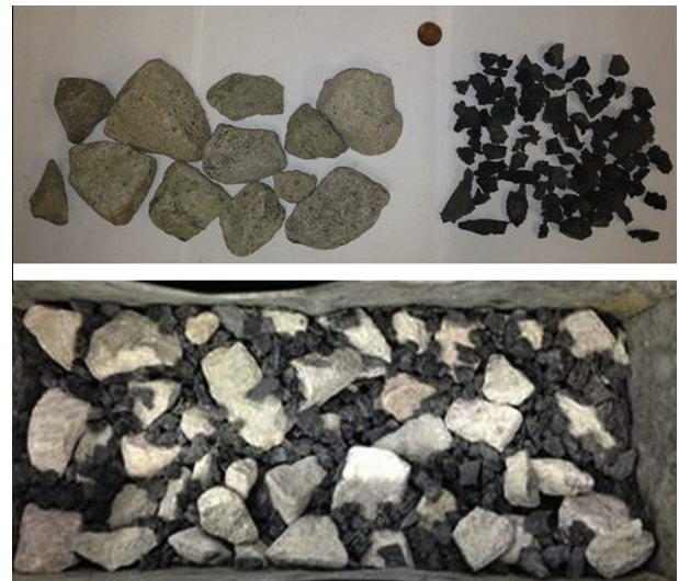
Fig. 1. Visual appearance of the ballast and crumb rubber used as well as the mix of both materials.
