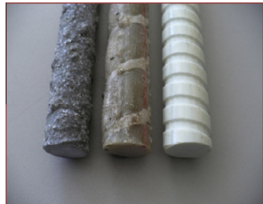
Fig. 1. Pultrall V-Rod, Hughes Bros. Aslan 100 FRP, and Schöck ComBAR (Left to Right) [5].
