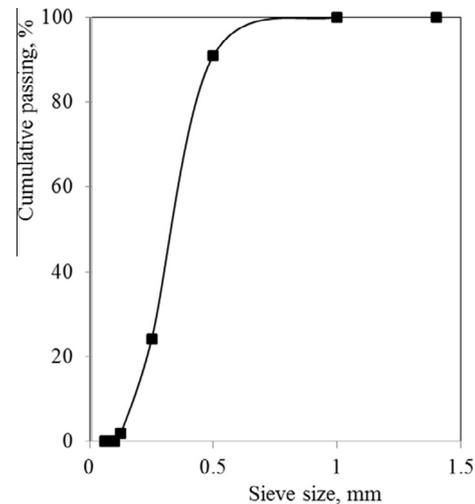
**Fig. 1.** Grain size distribution of the siliceous sand.
