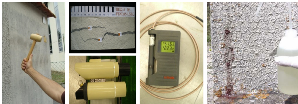
Fig. 1. Example of expedient tools used: from left: hammer tapping; crack width microscope measure (down) and crack width gauge (up); thermo-hygrometer; sodium hypochlorite solution.
