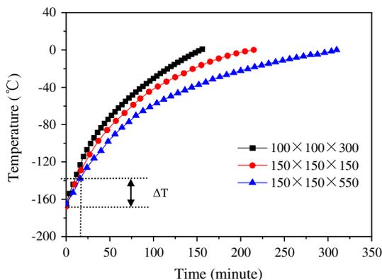
**Fig. 1.** Temperature rebound without cold insulation at the center of the specimens with different sizes (the legend is for the specimen size/mm × mm × mm).
