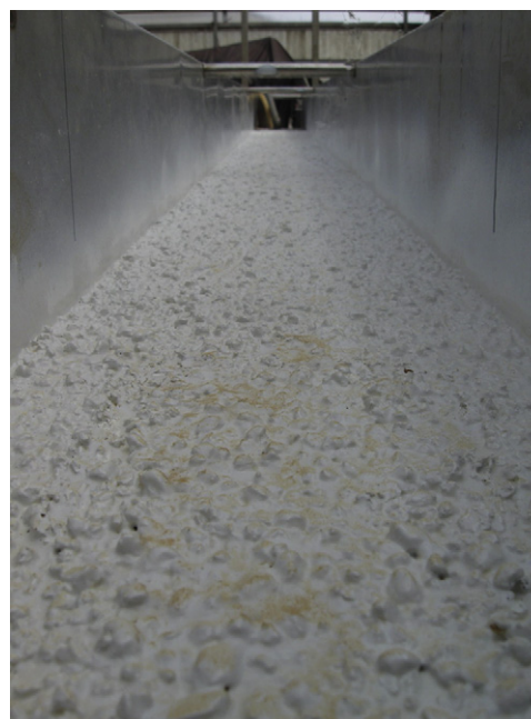
Fig. 1. Destruction of soil aggregates measured in a laboratory flume with constant roughness.
