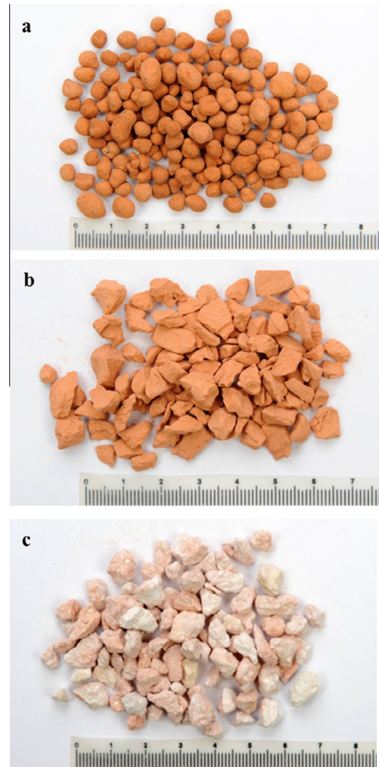
Fig. 1. Appearance of the investigated aggregates: (a) AC – granulated, (b) B0 – crushed, and (c) B5 – crushed.
