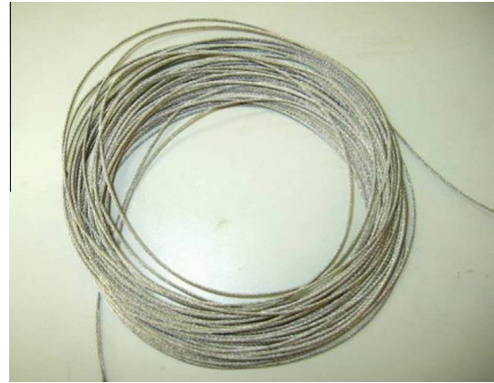
Fig. 2. High strength steel wire (HSW).
