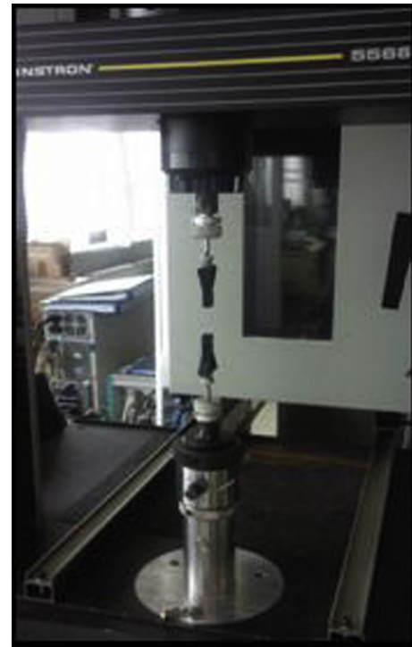
Fig. 1. Loading device for the tensile test.
