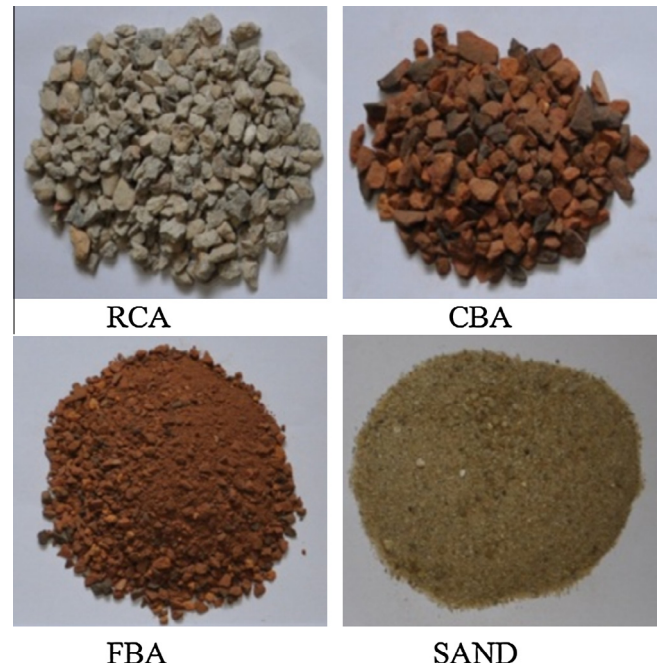
Fig. 1. Photographs of recycled and natural aggregates used in this study.
