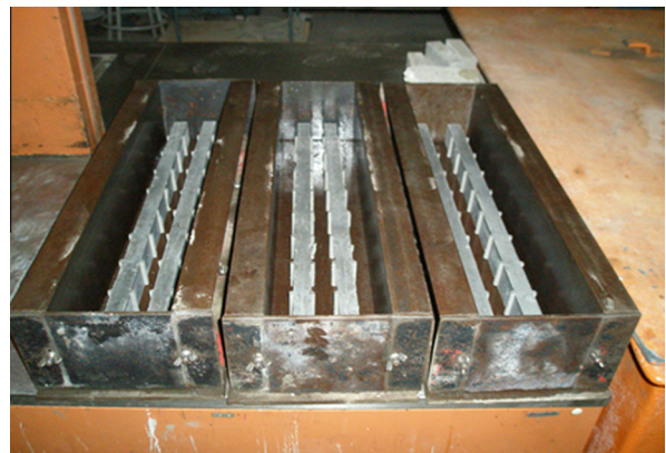
Fig. 2. UHPC bars in a mold prior to concrete placement.
