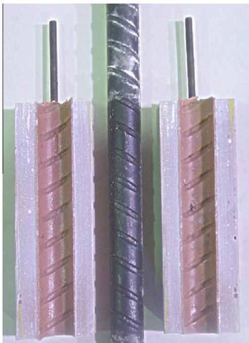
Fig. 1. Resin bolt separation after post-examination, after Aziz and Webb [2].
