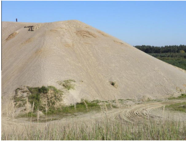
Fig. 1. Waste sand – a by-product of hydroclassification process of all-in-aggregate (photo by J. Katzer).
