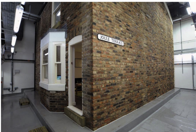
Fig. 1. The Salford Energy House within its environmental chamber.
