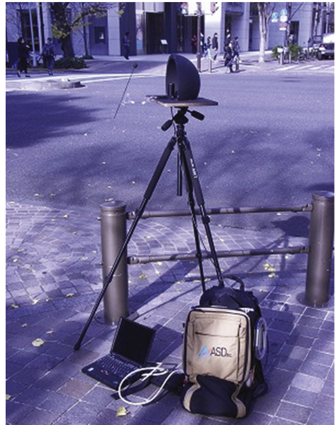
Fig. 1. Appearance of on-site measuring system.
