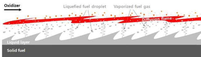
Fig. 1. Combustion mechanism of paraffin-based liquefying solid fuel.
