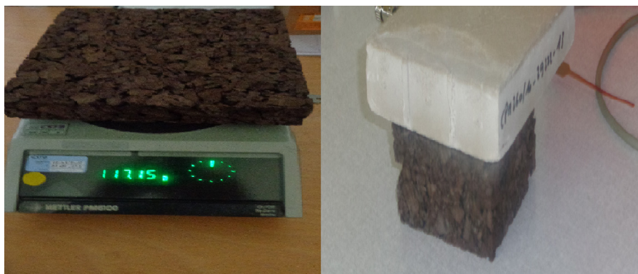
Fig. 1. Photos of black agglomerated cork tested specimens.
