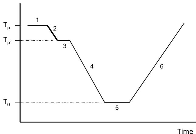
Fig. 2. Experimental protocol in the form of a temperature-time diagram for a thermostimulated depolarization currents experiment. The width of the polarising window is  $\Delta T = T_p - T_p'$ . In a partial polarization (PP) experiment it is typically between  $0$  and  $5^\circ\text{C}$ . The electric field is on in steps 1 and 2 (thicker lines). The depolarisation current is measured during the constant rate heating process (step 6).
