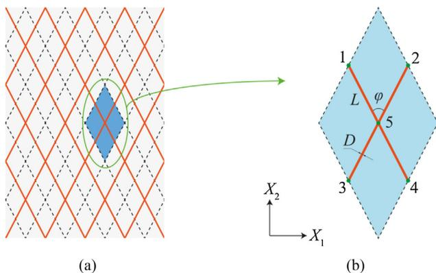
Fig. 1. Schematic illustrations of (a) the periodic mesh structure, and (b) the geometry of the RVE. The solid lines delineate the mesh structure, and the dashed black lines RVE boundaries.
