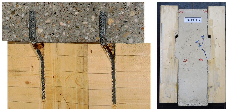
Fig. 1. Tested TCC connection (a) Dowel type fastener; (b) Notch [15].
