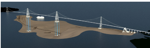
Fig. 1. Three-span suspension bridge with two floating pylons. Illustrated by Arne Jørgen Myhre, Statens vegvesen.
