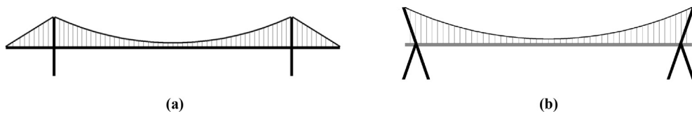
Fig. 1. Suspension bridge: reference design (a), modified design (b).
