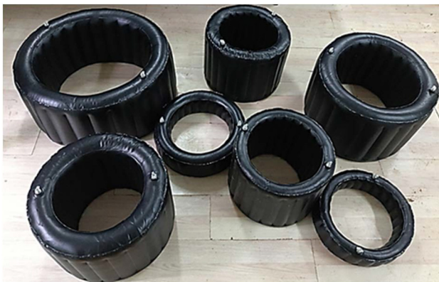
Fig. 3. Seven hollow cylindrical water barriers in the soft PVC containers.
