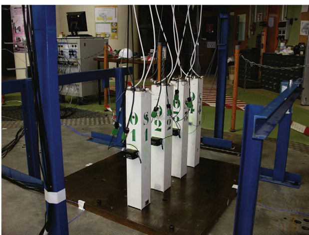
Fig. 1. The four tested blocks placed on the shaking table.
