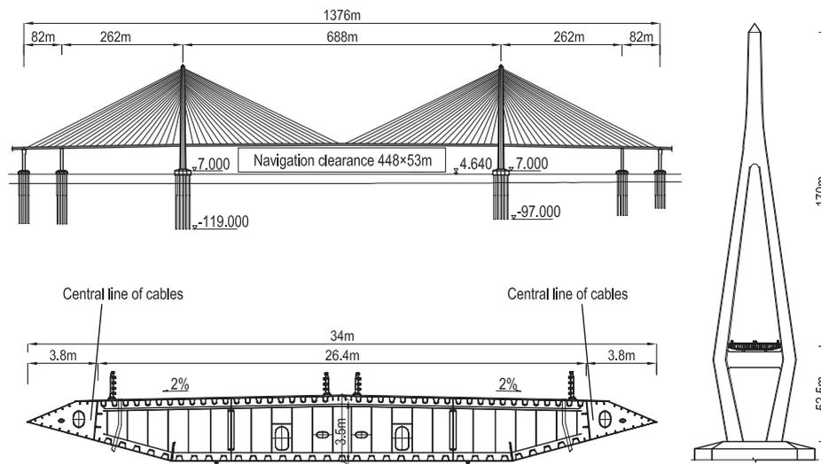
Fig. 1. General characteristics of Xiangshangang Bridge.
