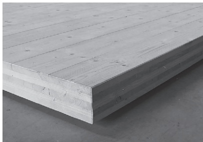
Fig. 1. (above) Principal CLT layup and some definitions of geometry and execution; (below) typical five-layer CLT element.
