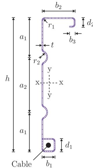
Fig. 1. Reference cross-section profile of the studied prestressed cold-formed steel beam. External dimensions are shown;  $r_1$  and  $r_2$  are the internal radii of the corners and web stiffeners respectively. Note that the x–x and y–y axes shown are the strong and weak geometric axes of the cross-section respectively, and that in-plane bending about the x–x axis is studied herein.
