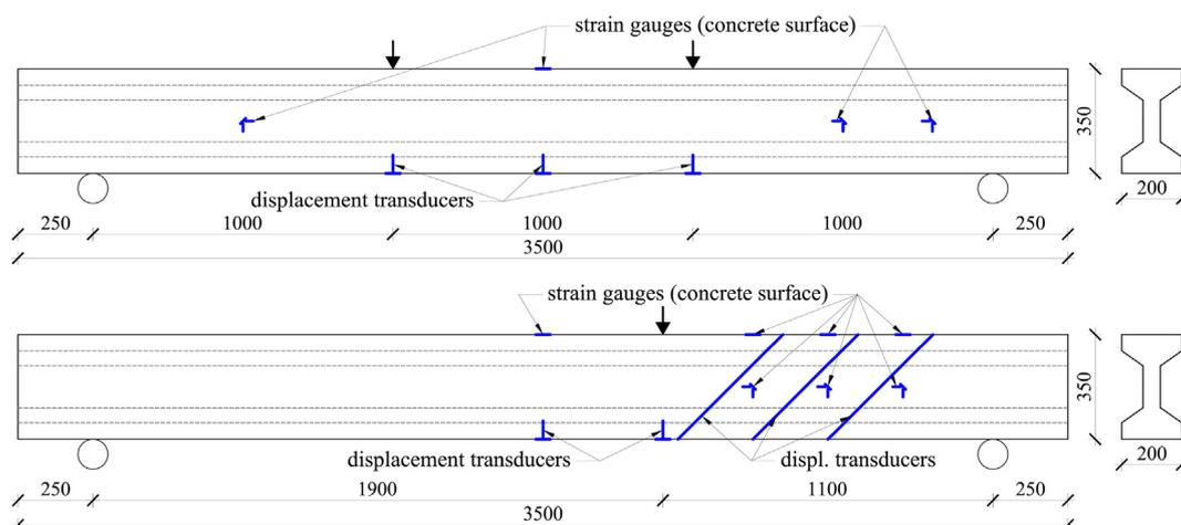
Fig. 1. Four-point and three-point test setups and external measurement devices.
