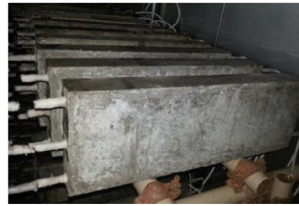
(b) Specimen in the marine environmental chamber
