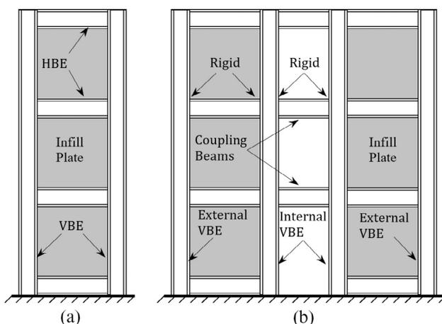
Fig. 1. SPSW systems: (a) conventional SPSW; (b) C-SPSW configuration.
