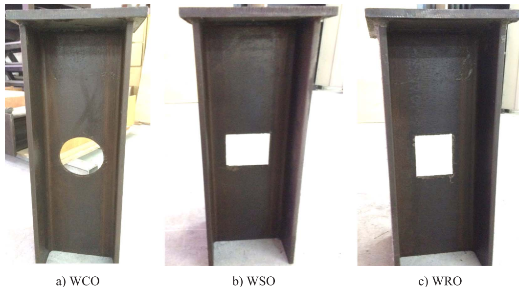
Fig. 2. Steel beam and opening configuration.
