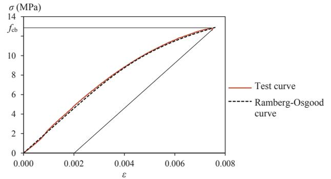
Fig. 2. Comparison between the measured stress-strain curve of the floorboard material and the Ramberg-Osgood material model.
