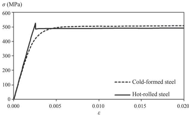
Fig. 1. Initial part of material stress-strain curves for typical cold-formed and hot-rolled steels.
