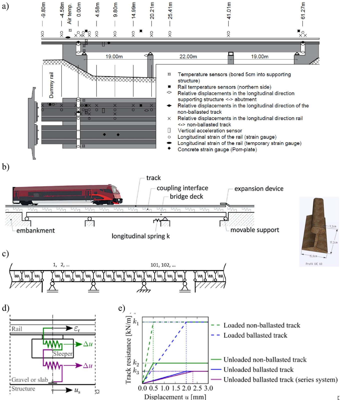
Fig. 1. (a) Static scheme and the monitoring systems of the L110 railway bridge (south view); (b) Spring-Beam model; (c) FEM Spring-Beam model; (d) rail structure interaction spring system for a singular supporting point; and (e) the track resistance – displacement model.
