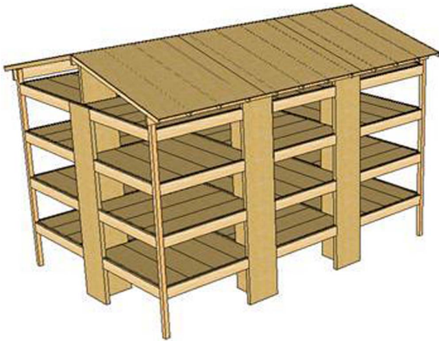
Fig. 1. Trä8 main components, including stabilising wall elements, in a multi-storey timber building [1–3].
